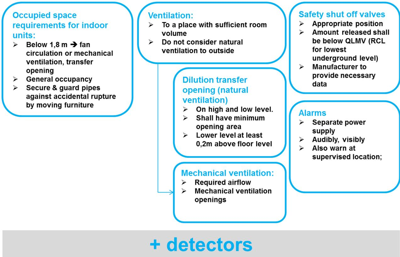
For other cooling systems such as chillers, the standard remains the same and there no restrictions other than chillers that are using A3 refrigerants and the limitations are as follows: -
